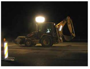
special events, parking lot lighting and other nighttime needs. Power is supplied by either a 120-volt outlet or a 2,000-watt generator. Each GloBug costs about \$3,000. Twenty GloBugs are in use on the 61/2-mile-long I-55/I-72 construction project.
