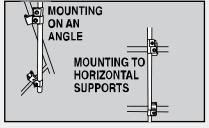
Flexible Clamps allow installation at any angle.
